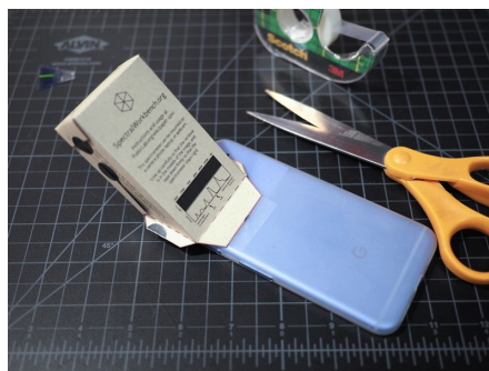
Fig. 4.1: Completed spectroscope attached to a phone.
